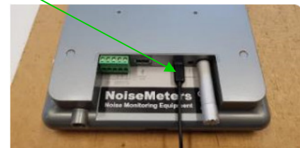
Fig 3: Mini USB end of mains power plugged into the SE3IND
